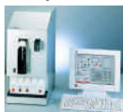
Fig. 2 Picture of Cedex® instrument along with the analyzing desktop computer. This system analyzes a sample's cell density and viability in 5 minutes.
